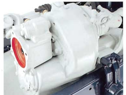
Fast pto for implements with high speed of revolution
