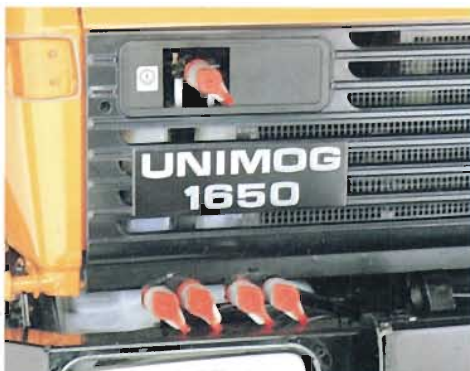
Up to 8 hydraulic connections each are possible front and rear
