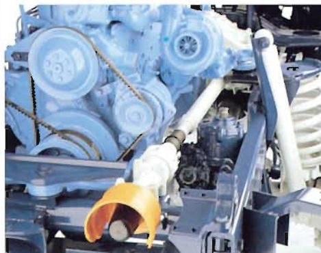
Pto stub shaft, 1 \frac{3}{8} " or 1 \frac{3}{4} ", splined/involute profile
