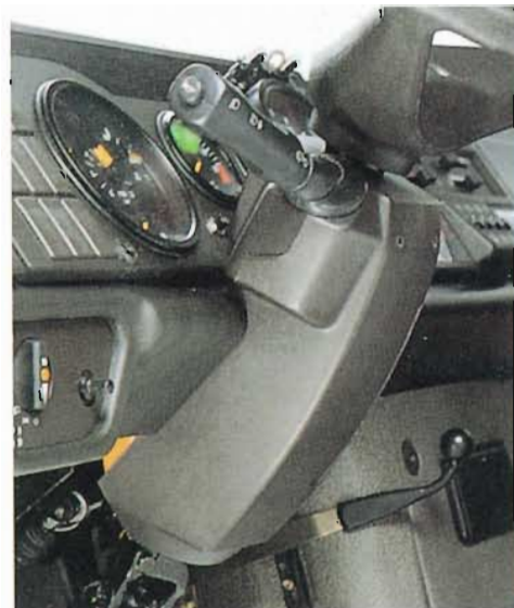
The steering column with redesigned plastic lining for greater safety
