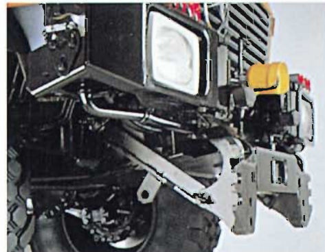
Implement mounting plate for easily attaching and removing front-mounted equipment
