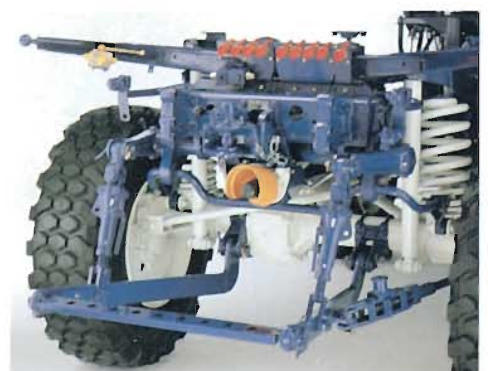
3-point rear power lift for heavy implements
